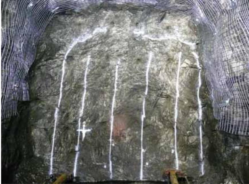
**Figure 1:** Massive sulphide with an average grade of 6.2% nickel exposed in a 5.2m wide ore drive at T1.
